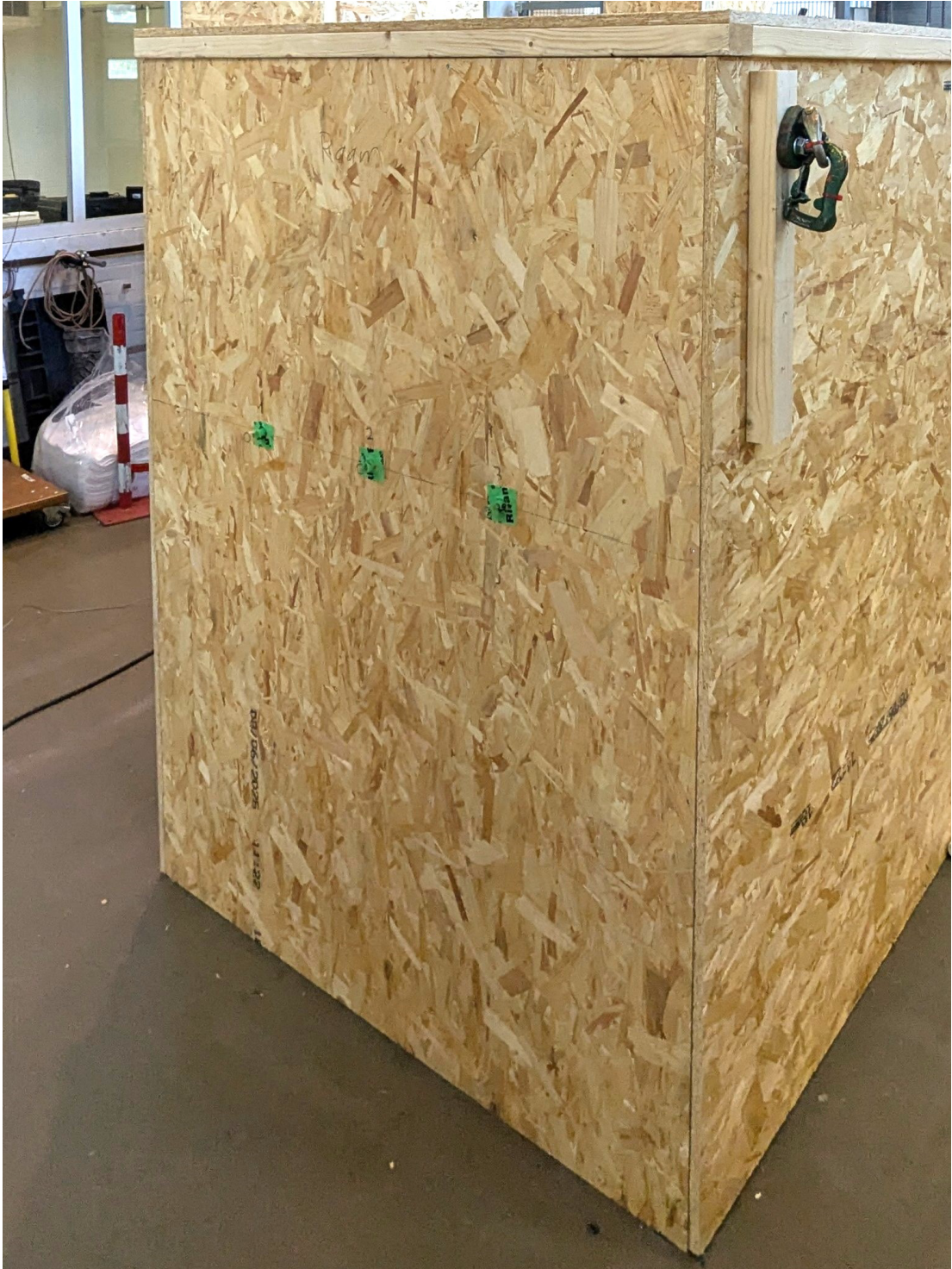
Figure H.13.: Sensor locations for measuring flow in the flow shield, for Vault 1 and 2. (1, 2, 3, left to right)
