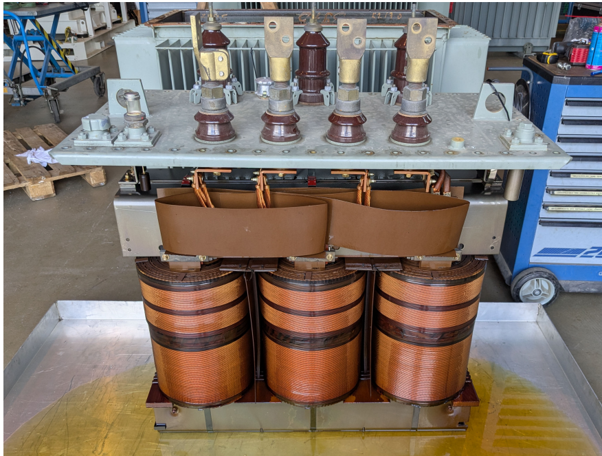
Figure 4.2.: Removed transformer internals for measurement.
